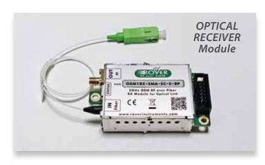
These compact OEM modules are very well shielded and specially designed for **Wireless Cameras** and **Microphones in the Broadcast world**.
