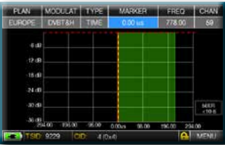
Fig. 1: OPTIMUM RECEPTION:* no ECHO present either outside or inside the guard interval mask (green area).
