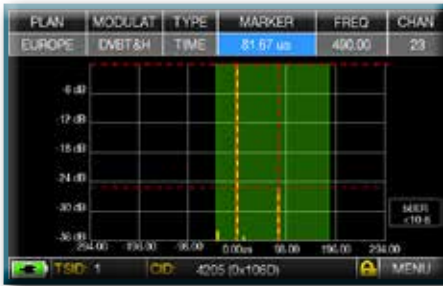
Fig. 2: GOOD RECEPTION:* 2 ECHOES present, but within the guard interval mask (green area) coming from a distance of: 1st echo: 24,50 Km, the same as a 81,67 \mu s delay.
