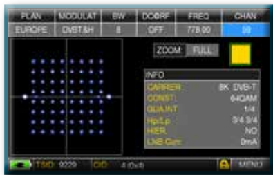
Fig. 4: DVB-T-64Q CONSTELLATION: The table to the right shows all the received modulation parameters
