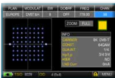
Fig. 4: DVB-T-64Q CONSTELLATION: The table to the right shows all the received modulation parameters
