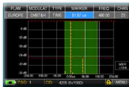
Fig. 2: GOOD RECEPTION:* 2 ECHOES present, but within the guard interval mask (green area) coming from a distance of: 1st echo: 24,50 Km, the same as a 81,67 \mu\text{s} delay.
