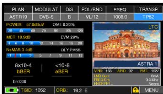
Main measures and image of a SAT signal.
