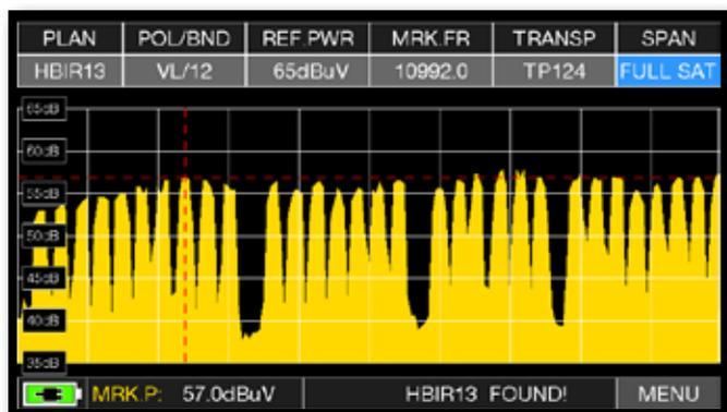
SAT spectrum SPAN "Full SAT"
