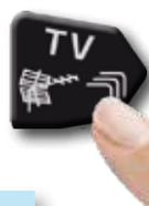
Press repeatedly to navigate into TV measures screens: Measures, Constellation, echoes and MER vs CARRIER.
