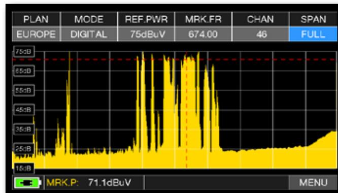
"TV" SPAN FULL spectrum (from 30 to 1.000 MHz).
