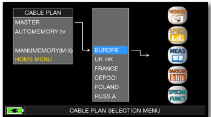
Touch directly the decided canalization or use the encoder. At the end touch "MEAS" to make the measure or "SPECT" for visualize the spectrum.
