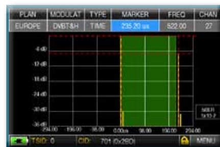
Fig. 3: MARGINAL RECEPTION (or IMPOSSIBLE):* 2 ECHOES present outside the guard interval mask (green area), coming from a distance of: 1st echo: 70,56 Km, the same as a 235,20 \mu\text{s} delay.
