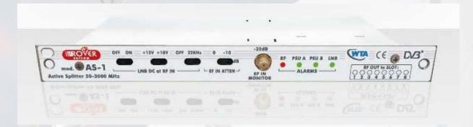
**AS1** = Amplifier module with 1 input and 4 outputs, Freq. range 50-3000MHz, input rf power sensor, -20dB monitoring port, deep switch to manage the LNB power supply output (OFF/13/18V, 0/22KHz) and a deep switch to add 10 dB attenuation on the output. Maximum 4 modules per rack.
