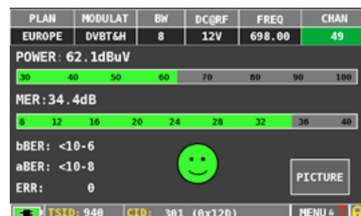
Screen showing DIGITAL TV signal measurements
