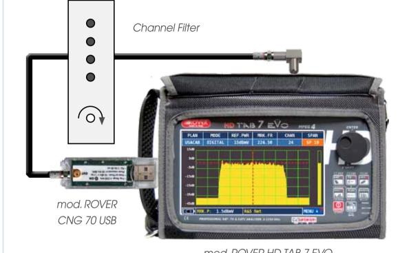
How to connect the CNG 70 USB to a distribution network:
