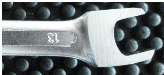
**Picture 1b: Wrench key n.13.** This picture shows a modified wrench (planed head) we use in our production to make it easier to access difficult points to tightening the nuts. This is just for information; **this tool is not included** with the HW kit of this app.
