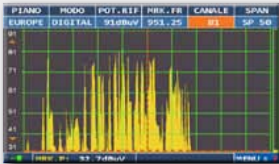
FIG. 1 reception power measurement in the 935 to 960 MHz band
