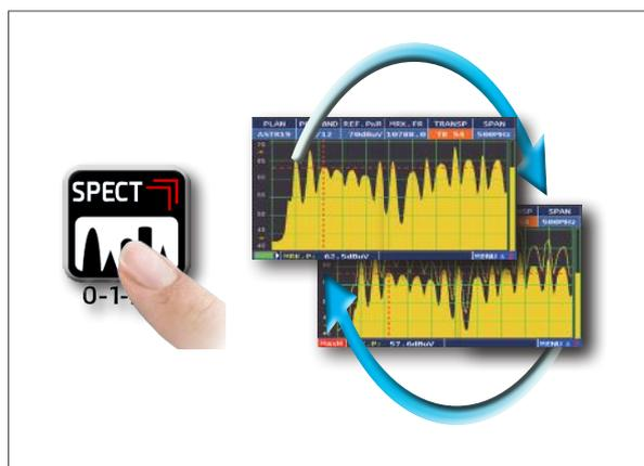
Press to cycle through the spectrum analyzer screens
