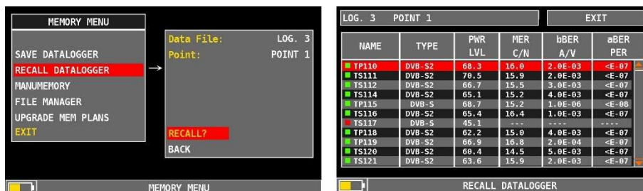
Fig.6 Logger results. The main measurements (not all) will be displayed. The amber and red small squares indicate a measurement which is not inside the threshold of a PASS signal. To get the full set of measurements, download the logger to a PC or export this to an Excel file using the Rover SMART.
