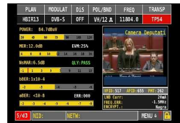
Fig. 10 when measuring in SCR mode, the user band shows on the bottom left side of the screen
