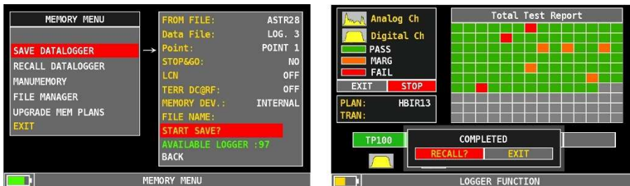
Fig.5 Logger in progress with the corresponding measurements results. At the end of the logger the meter will ask if to display the logger results.
