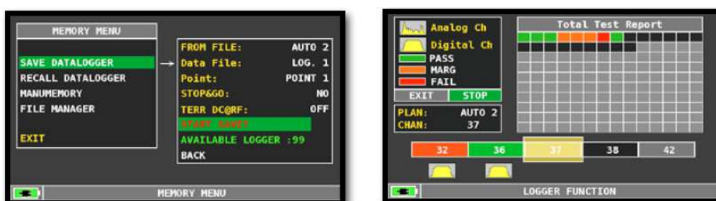
Fig.5 Logger in progress with the corresponding measurements results. At the end of the logger the meter will ask if to display the logger results.
