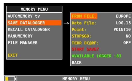
Fig.4 Select the Save DATALOGGER entry.
