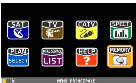
Fig.3 Main menu, select the MEMORY icon to start the logger function.
