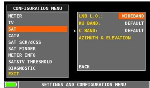
Fig.7 Wide band setup in the configuration menu.
