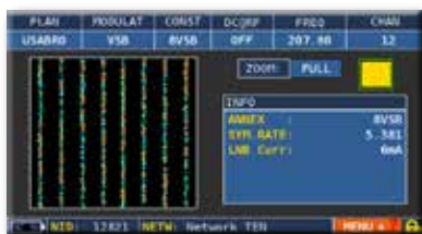
VSB constellation, on the right relative modulation parameters
