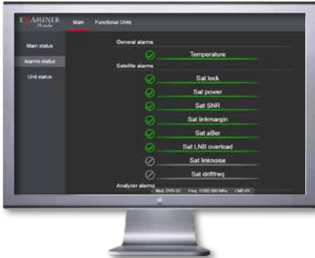
General status with the main alarms in one screen.
