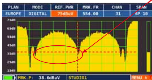
FIG 2. REFLECTION MEASUREMENT (ECHOES)
