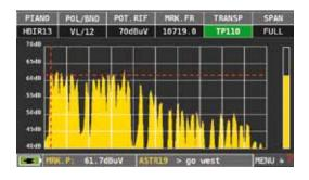
direction. When you have finished pointing the dish, the lower part of the display shows the words "HBIR13 FOUND!". Depending on the diameter of the dish used, moving the dish in a range of  $\pm 10^\circ$  according to the chosen satellite, the instrument will show, each time, in Full Sat Expert spectrum mode, which satellite you are pointing at.
