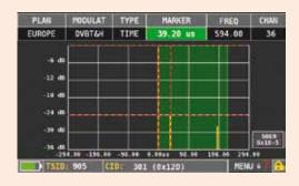
is shown on the instrument by a green band of colour, this also helps the installer to understand if an ECHO is located inside or outside the Guard Interval.
