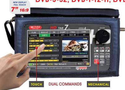
ROVER'S new HD TAB 7 is a COMBINED PROFESSIONAL HD TABLET ANALYZER, 4-2.250 MHz for SAT QPSK/8PSK, TV COFDM (T2 M-PLP opt.) and CATV QAM (C2 opt.), with MPEG-2/4 decoder, Analog TV & Radio; it has a TABLET format and is extremely small and light (only 4 cm thick and weighing 1.6 kg).
