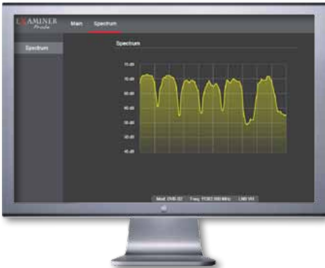
Spectrum analysis with selectable SPAN.
