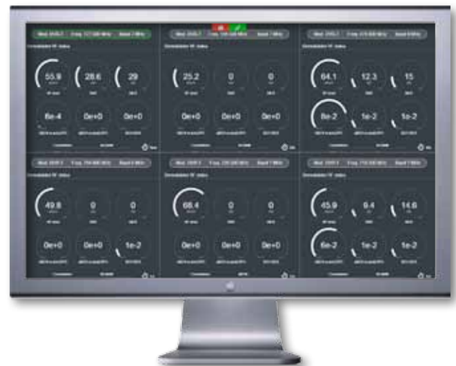
It scans the network at the selected frequencies in any modulation in round-robin.
